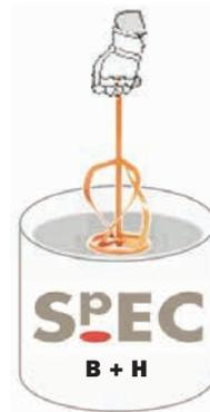
The components should be mixed for a minimum of 5 minutes to obtain a uniform colour, free from streaks. Mixing should take place using a slow speed drill (300-400rpm) fitted with a **SpECseal** paddle mixer.
