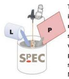
The liquid should be poured into a 20 litre plastic or metal drum. The powder should be added slowly whilst mixing with a spiral paddle attachment on a slow speed electric drill.
